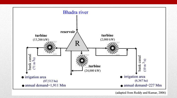
• The **Bhadra dam** is situated in Chimagalur district of Karnataka state, India. The reservoir provides water for irrigation of 87,512 ha and 6,367 ha. There are three Hydropower turbines. One turbine is at the bed of the dam. Data of monthly inflows were notably collected over a period of 69 years.
